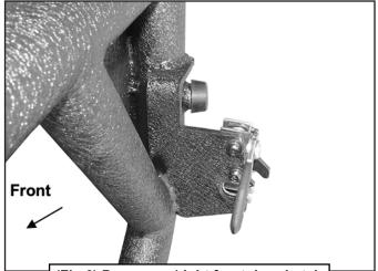
(Fig 6) Passenger/right front door Latch and Rubber Bumper installed
