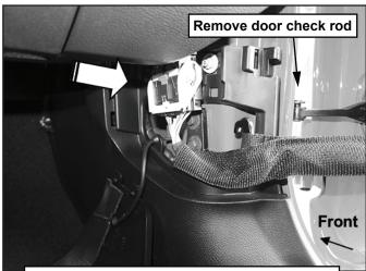
(Fig 3) Remove cover and unplug wiring harness from under dash if equipped, (arrow). Release door stop strap and check rod
