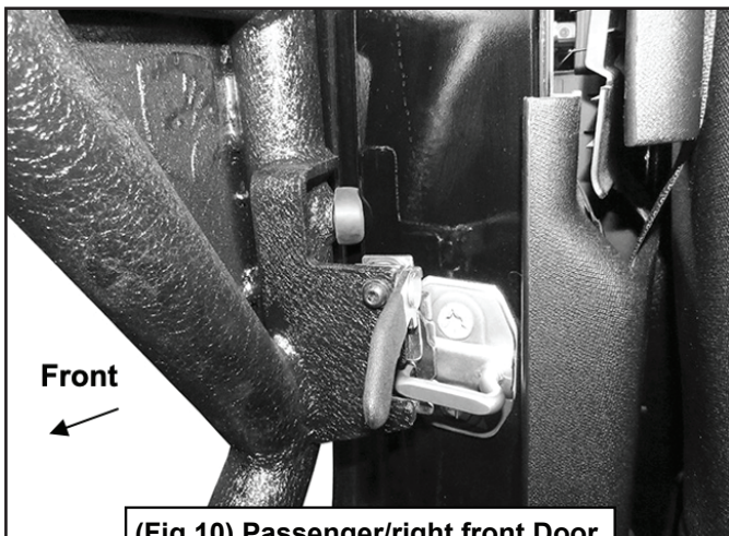
(Fig 10) Passenger/right front Door with Bumper and Latch installed
